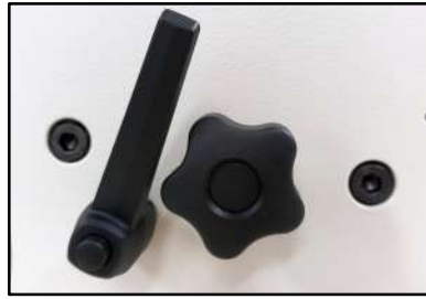
Many possible setups to adjust the parallelism of the press for an uniform closing of the Wire-O® binding
