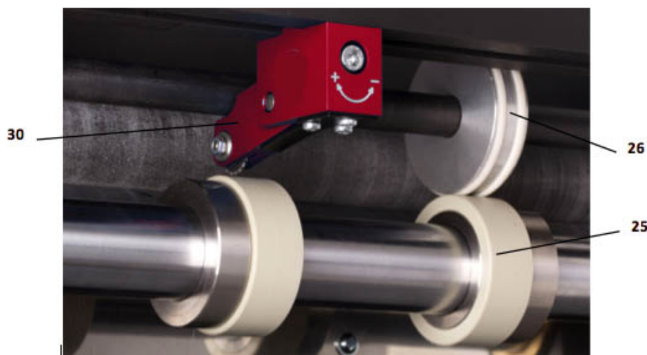
Fig. 11: Setting Rotary Perforating and Cutting
