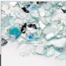
Particles of shredded CDs, DVDs, Blu-ray discs Cutting size 20 x 40–50 (1,000 mm 2 )
