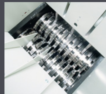
Cutting unit stage 1: Pre-shredder
